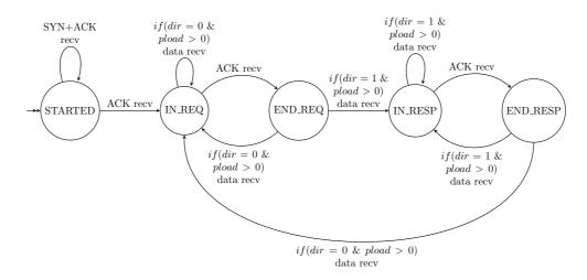
Figure 2 EFSM used to model a TCP-based request-response protocol.
