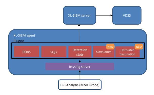
Figure 4. XL-SIEM plugin schema for the MMT Probe after the second iteration
